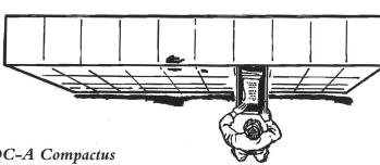
The BOC-A Compactus offers storage capacity equivalent to 10 four drawer filing cabinets and reduces the floor area dedicated to storage by up to half.
